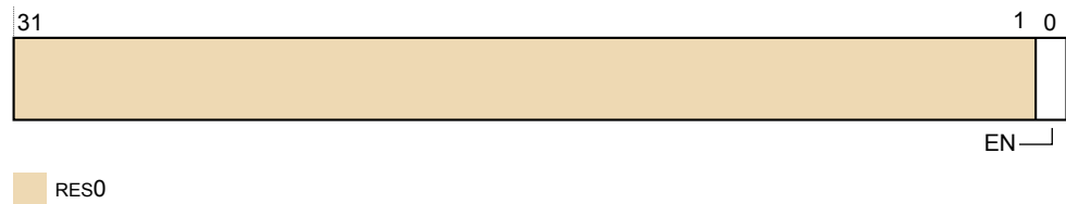
Figure D8-2 MUSERENR_EL0 bit assignments
